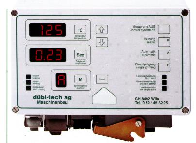
electronic hot-foil monitoring system with foil rupture control, pre-alarm for foil end on optical display, not any product leaves the production line unprinted (product liability)
